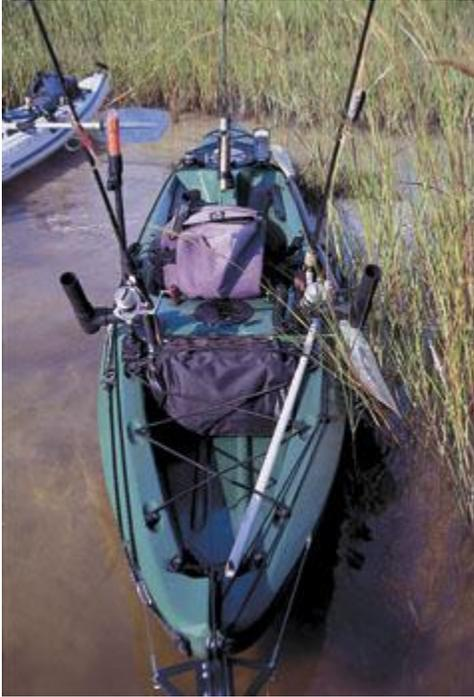
Oswald also recommends that fishermen purchase a kayak with a rudder. He uses the foot-operated steering device to control and steer his boat along shorelines when he's plugging with the wind at his back. On days the breeze kicks up to over five mph, he deploys a drift sock on the anchor trolley that allows him to crawl down fishy shorelines. Forward and rear bungee systems increase storage capabilities; they're also good for keeping PFDs close at hand.
