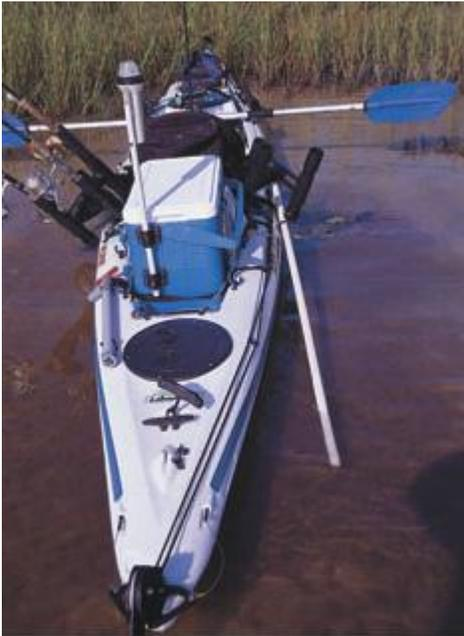
*This rig features a dry storage compartment, cooler with nav light, hand bilge pump for emergencies and PVC stakeout pole.*
